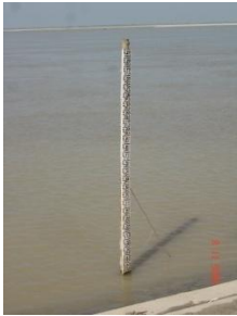
Figure: Water Level Gauge at Seraiganj on Jamuna River
